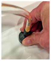
Choose the rubber suction cup that is correct for the fastener and washer size to be tested. The cup must clear the washer to the full perimeter.
